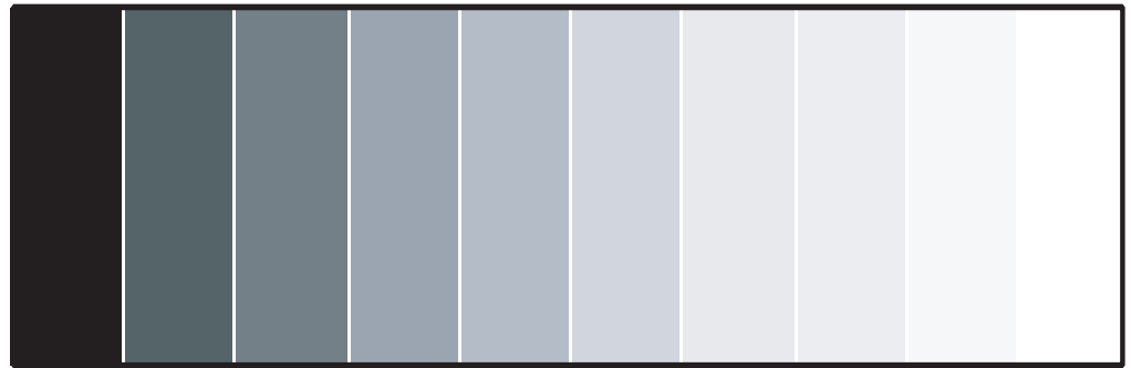
Figure 4-3. Typical Gray Bar Pattern for Adjusting Contrast
